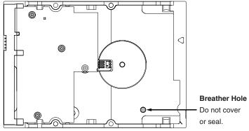
**Caution.** Do not cover, seal, or insert any object into this hole. This hole has two purposes:
